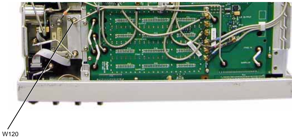
Placement of W120
